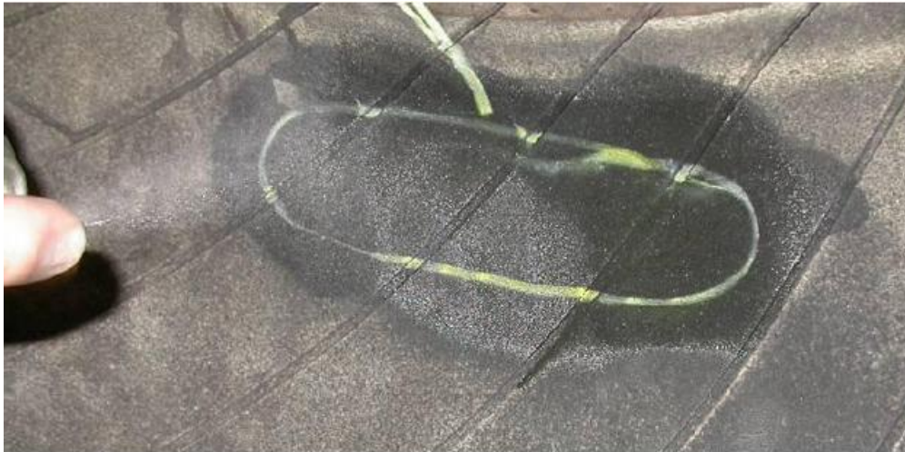
Applying cleaner fluid to the outlined area
